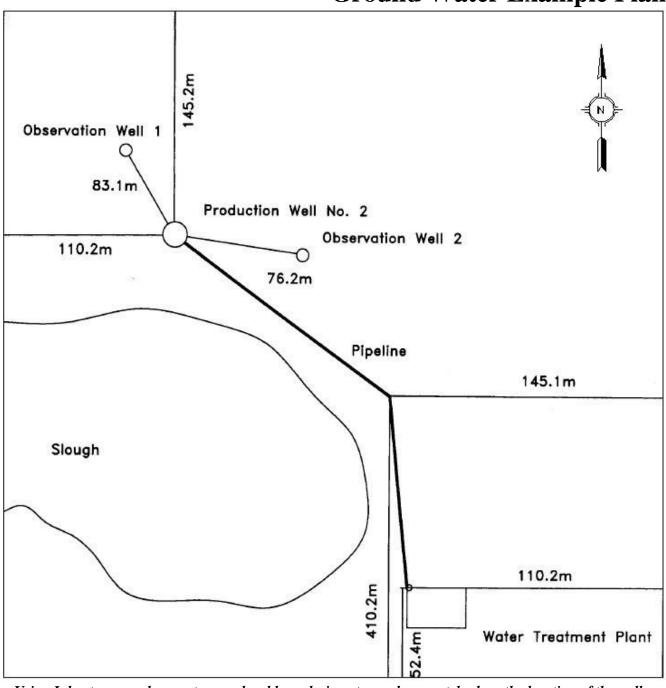
Using Ink – trace roadways, streams, legal boundaries, etc., and accurately show the location of the well, observation wells, pipelines and other works measured from legal boundaries.
