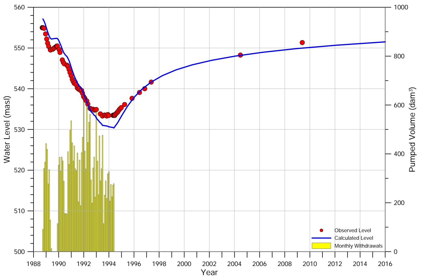
Figure B.27: Hydrograph and drawdown of well **M16R-84**
