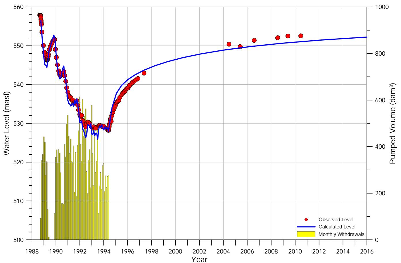
Figure B.11: Hydrograph and drawdown of well **M18UL-84**
