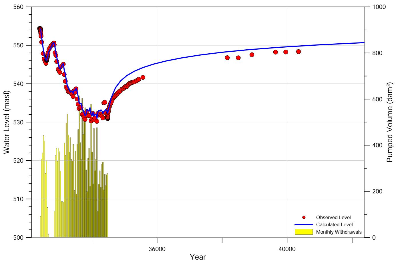
Figure B.18: Hydrograph and drawdown of well **M30UL-88**
