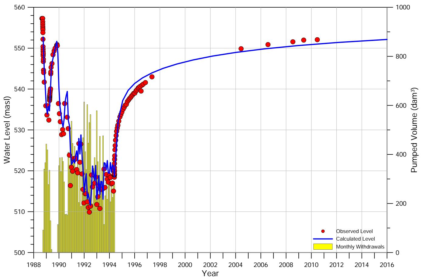
Figure B.9: Hydrograph and drawdown of well **M13UL-84**
