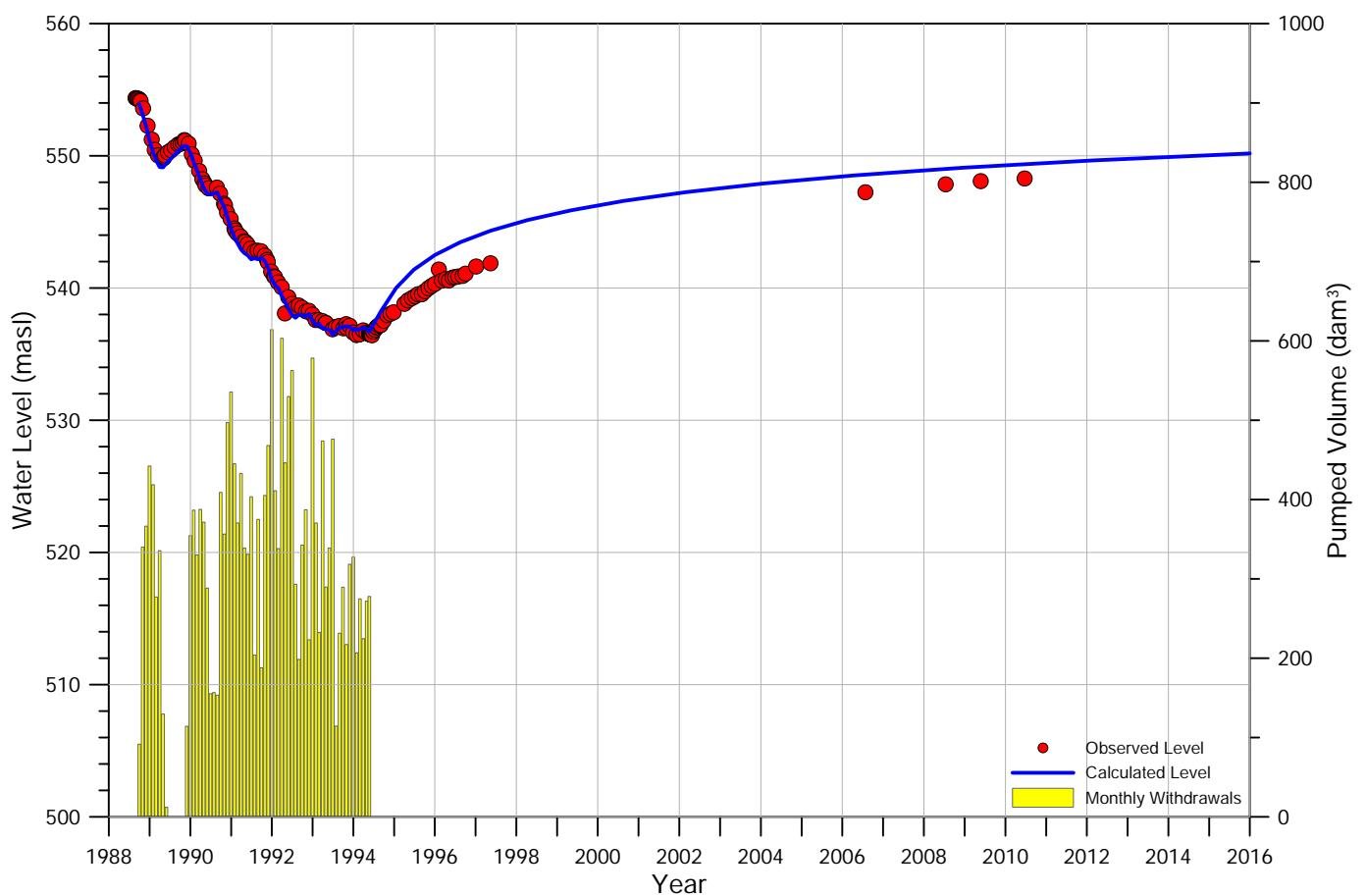
Figure B.1: Hydrograph and drawdown of well **GSC3AL-60**
