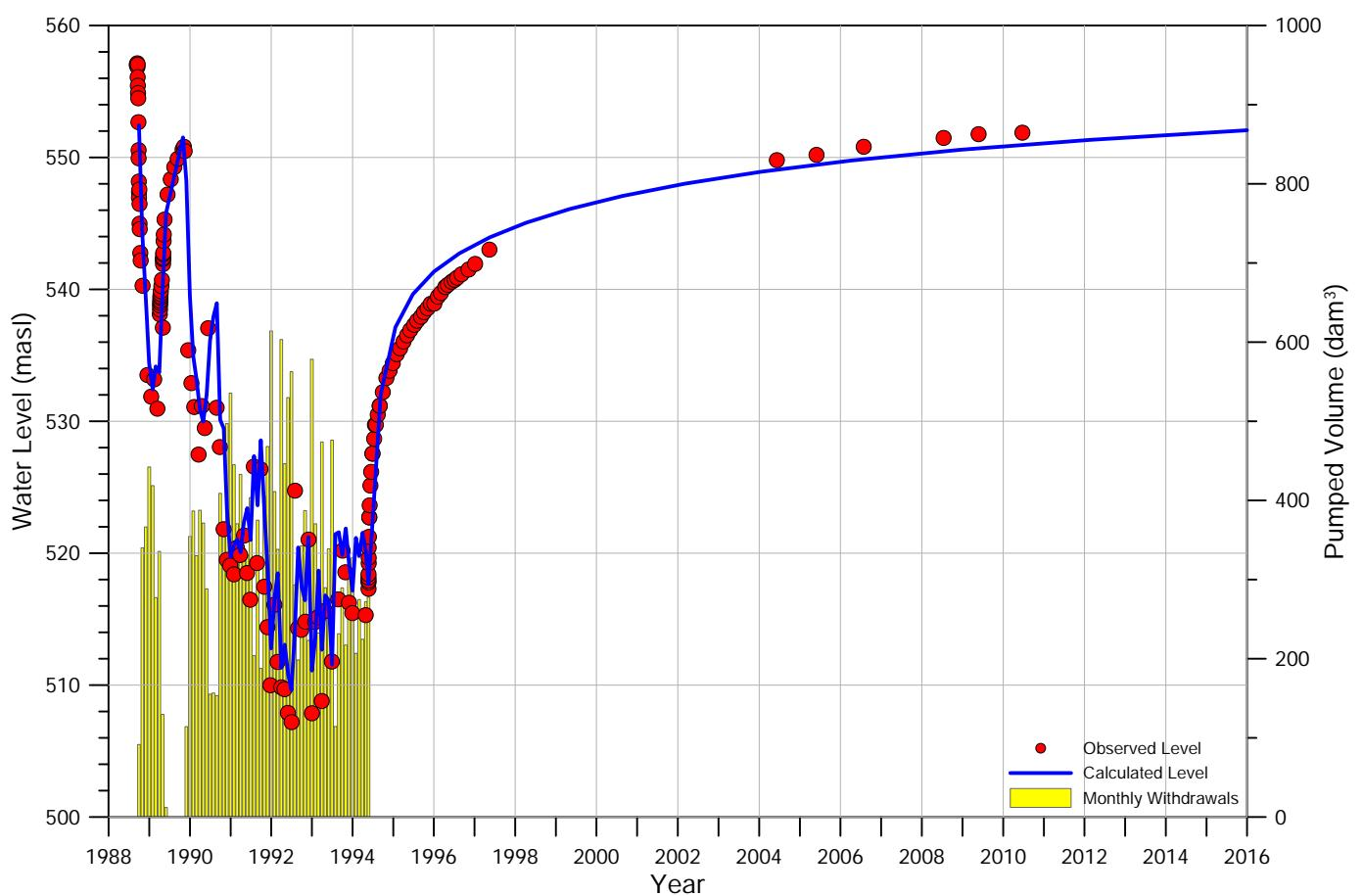
Figure B.15: Hydrograph and drawdown of well **M22UL-88**
