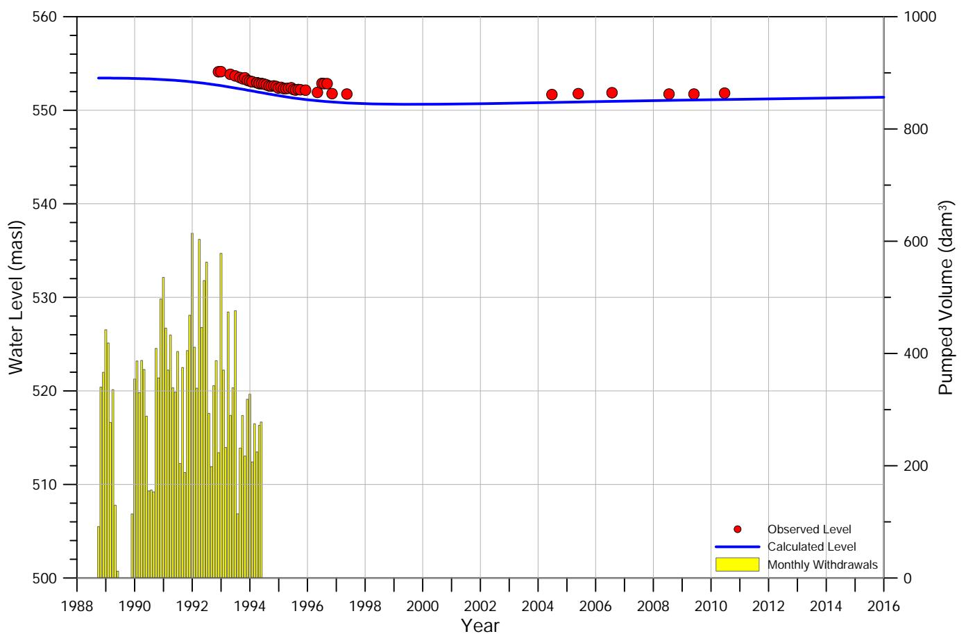
Figure B.29: Hydrograph and drawdown of well **M36R-92**
