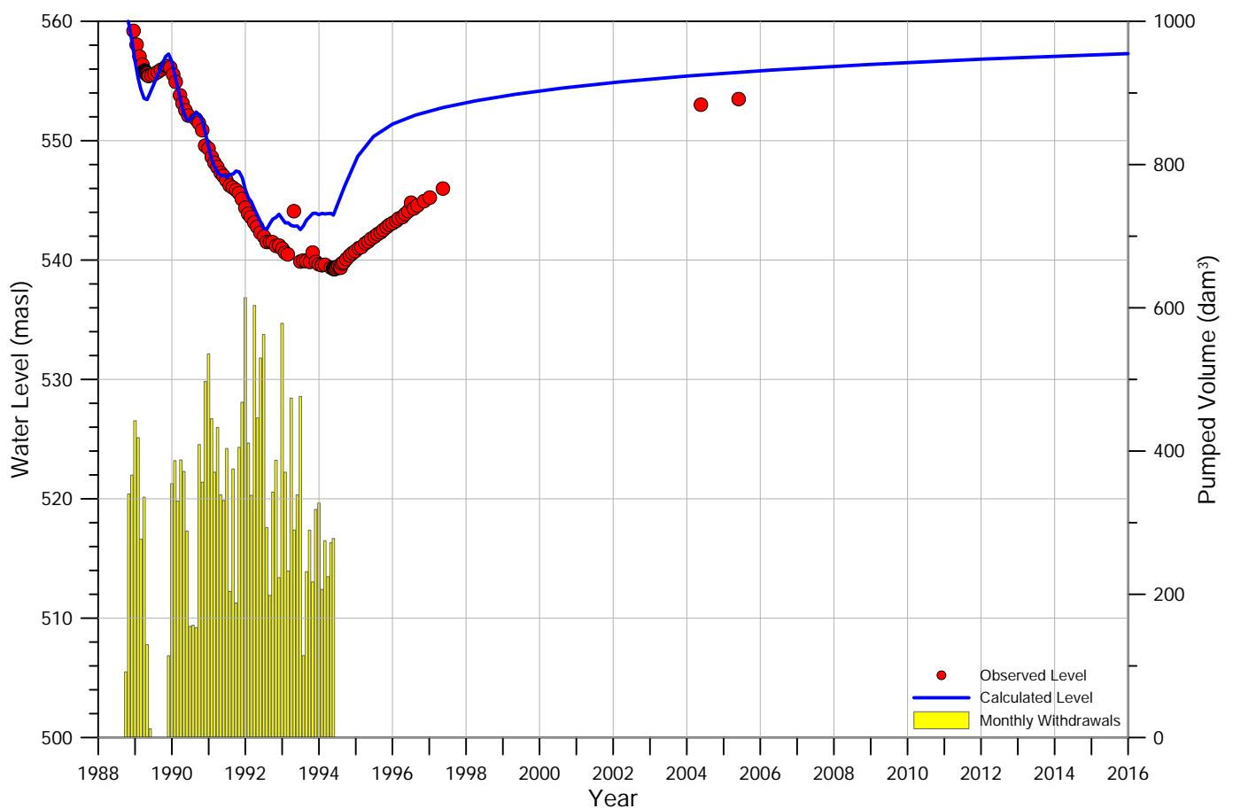
Figure B.17: Hydrograph and drawdown of well **M28UL-88**
