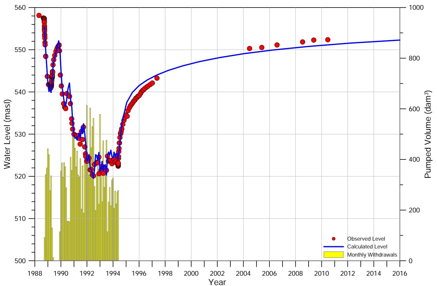
Figure B.7: Hydrograph and drawdown of well **M11L-84**
