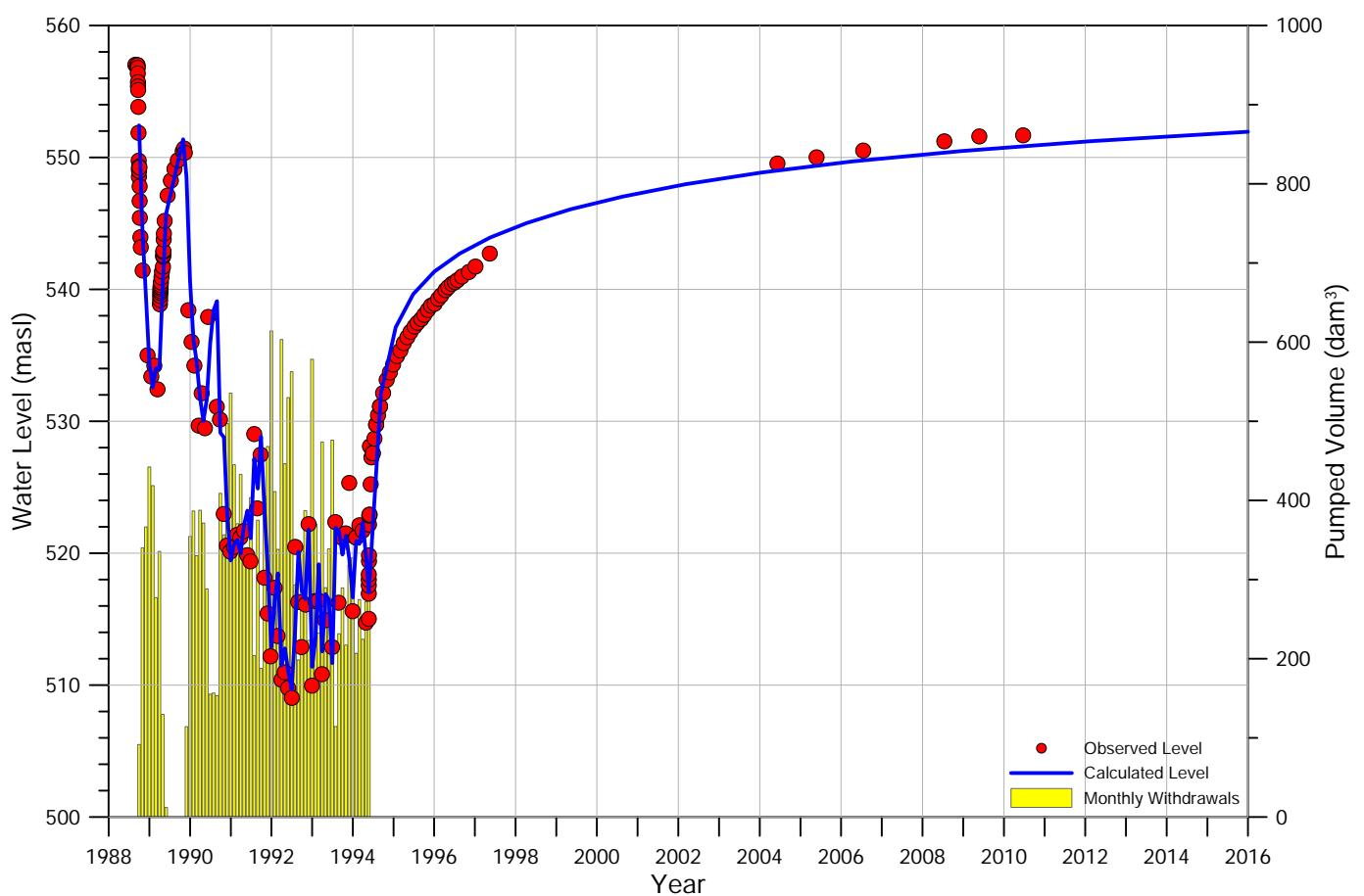
Figure B.12: Hydrograph and drawdown of well **M19UL-84**
