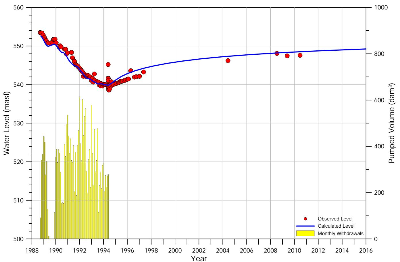
Figure B.22: Hydrograph and drawdown of well **R6UL-88**
