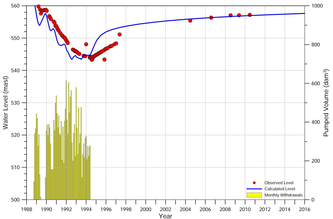
Figure B.21: Hydrograph and drawdown of well **R3UL-88**
