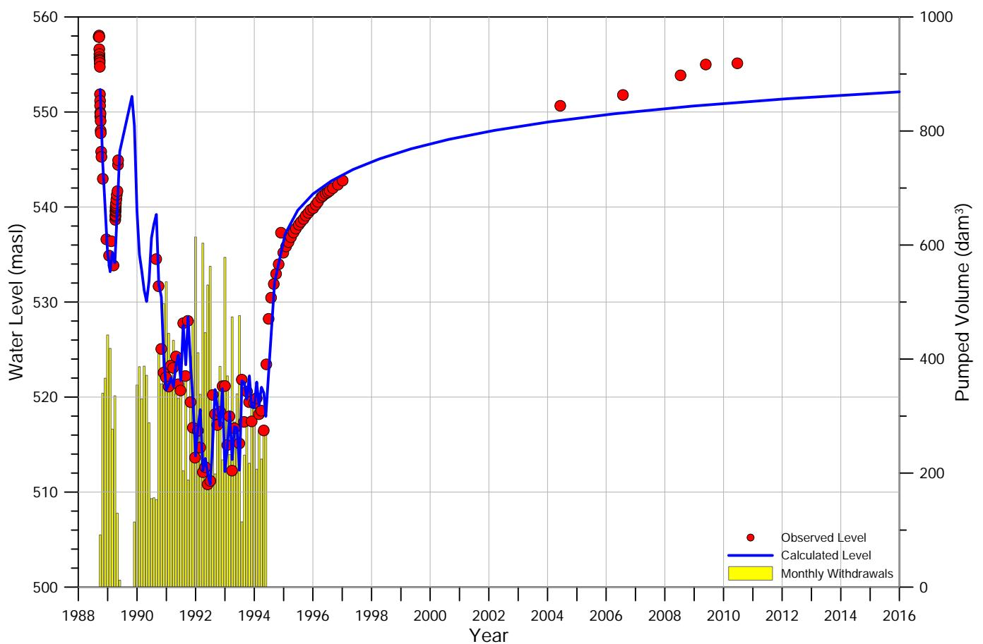
Figure B.14: Hydrograph and drawdown of well **M21UL-86**
