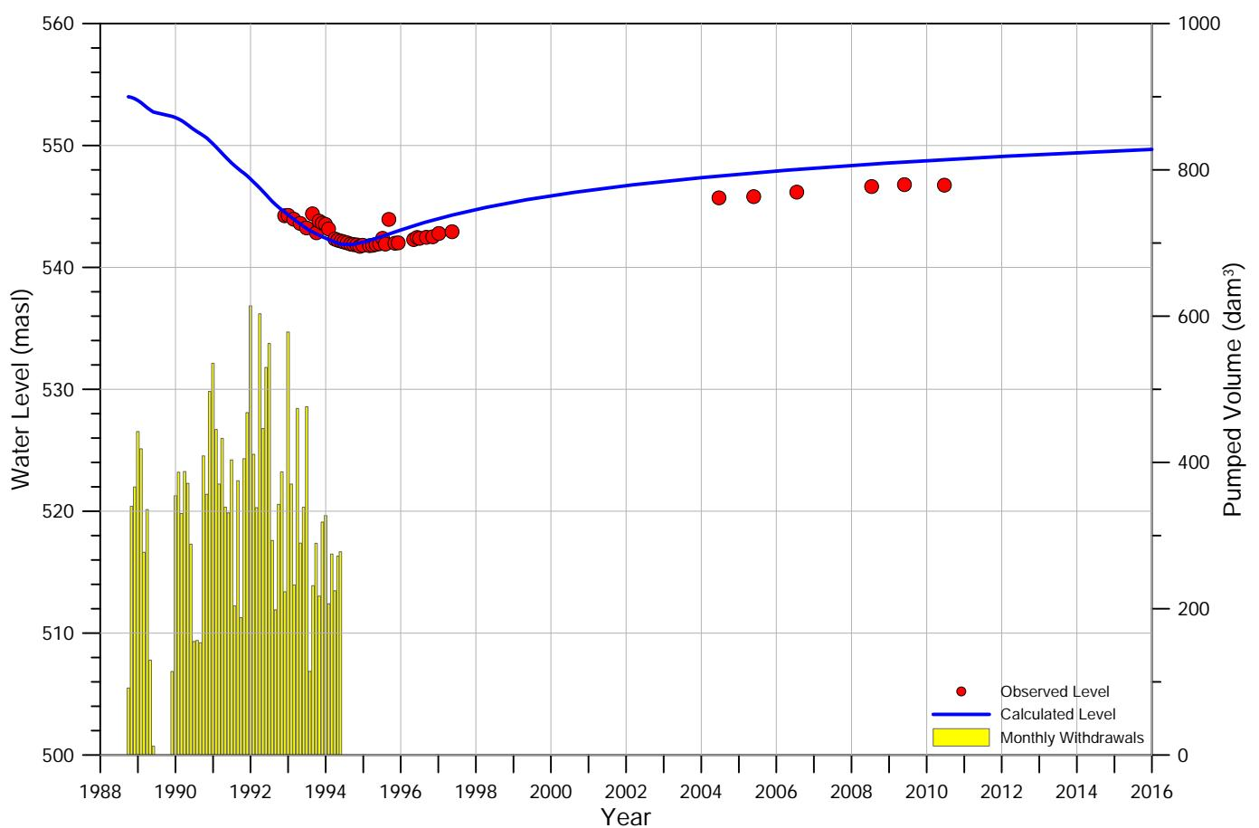
Figure B.28: Hydrograph and drawdown of well **M35R-92**
