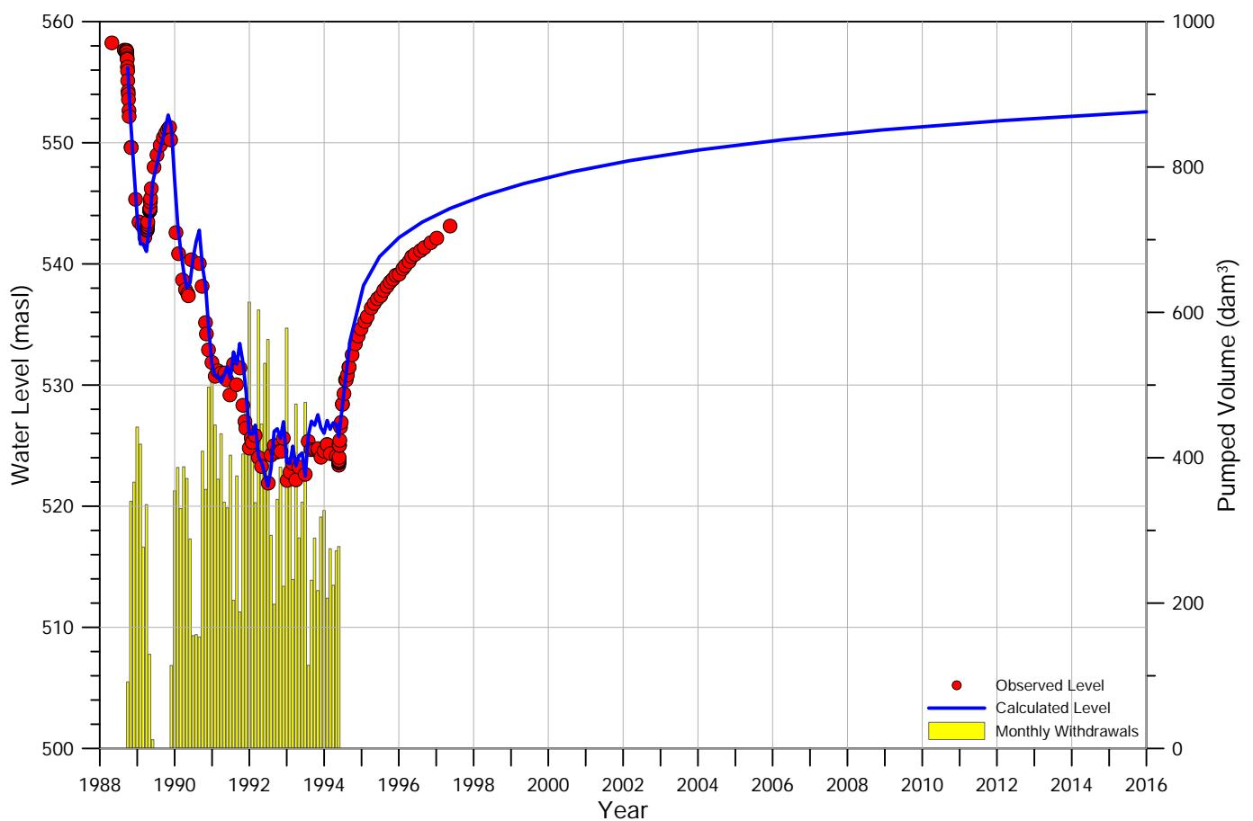
Figure B.3: Hydrograph and drawdown of well **M06L-82**
