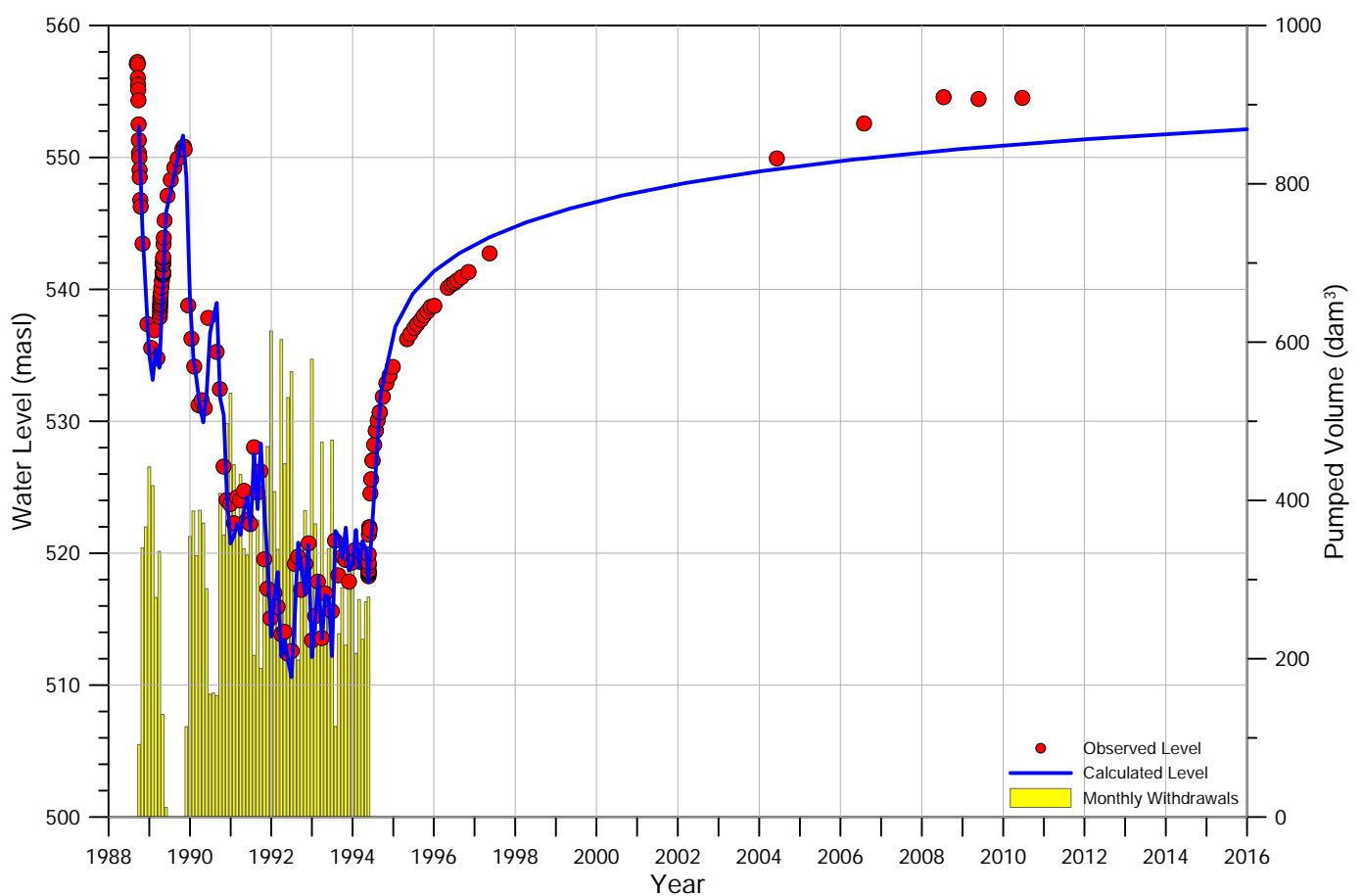
Figure B.5: Hydrograph and drawdown of well **M09L-82**
