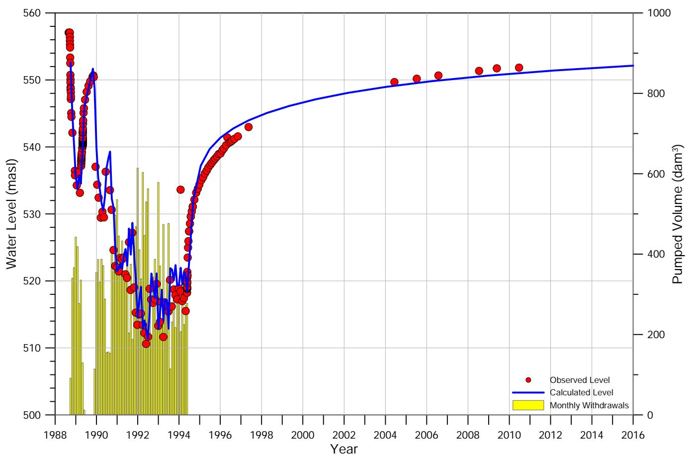
Figure B.8: Hydrograph and drawdown of well **M12UL-84**
