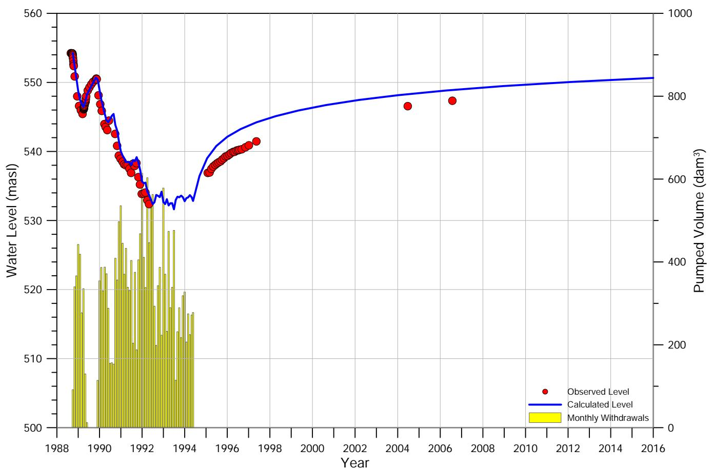
Figure B.24: Hydrograph and drawdown of well **TW1L-65**
